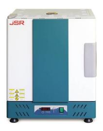
JSON-Series Dry Heat Sterilizer is a common instrument to be used to drying, heating and sterilizing objects by heating air up to +160 °C or +180 °C with gravity convection system during specified sterilizing exposure time range from 30 to 60 minutes.
