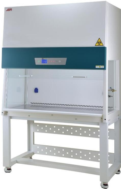
Vertical Laminar Flow Cabinet enclosure designed to maintain ISO Class 5 (formerly Class 100) clean air. HEPA filtered laminar air down flow over the work area to protect products or samples being handled in the cabinet from dust or biological contaminants such as bacteria, fungus and genetic materials.
