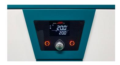
Dual Chamber Refrigerated BOD Incubator provides 2 x 250 liter chambers and each chamber has an individual temperature controller. 10 Steps of temperature programming as well as constant temperature operation range from  $+0\,^{\circ}$ C to  $+70\,^{\circ}$ C for more versatile use. It gives an excellent performance for incubation of microorganisms, BOD (Biological Oxygen Demand) Test and various QA / QC Tests.
